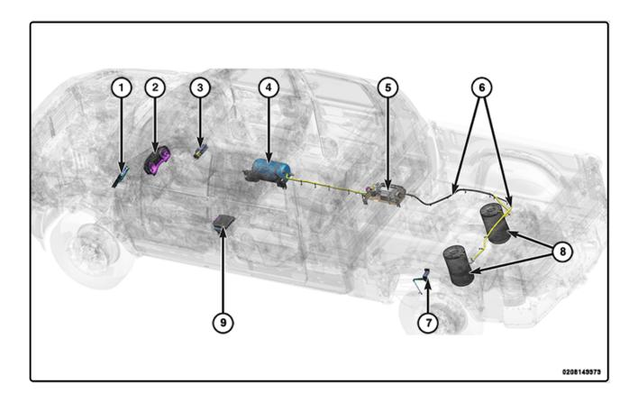
The air suspension system consists of the following major components:
