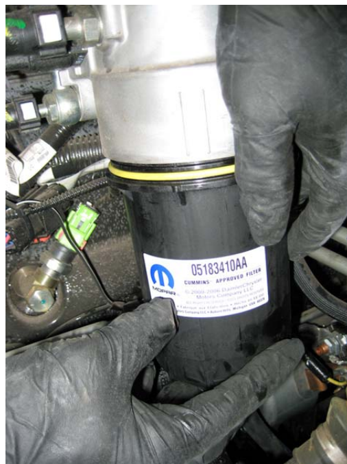
With one hand above and one hand below you can get to the fuel filter from above.
